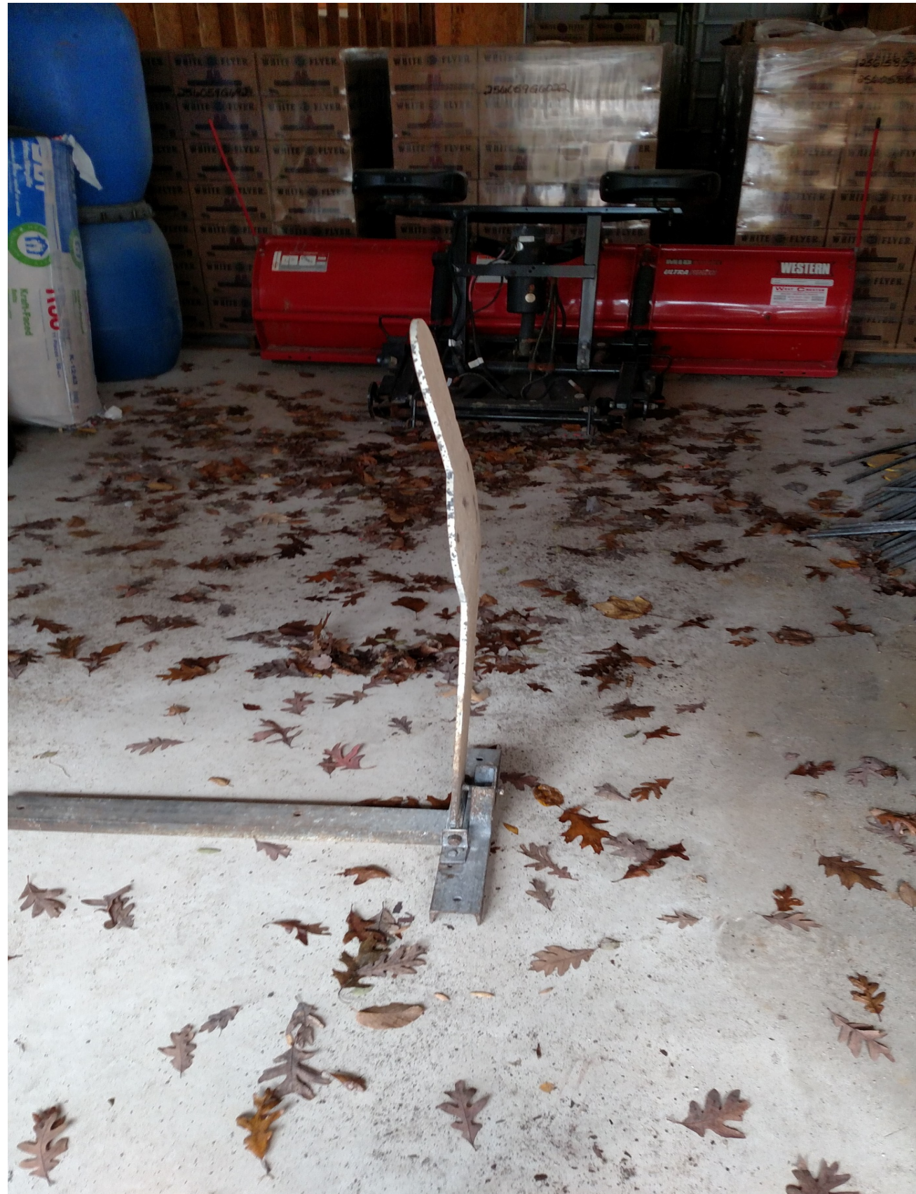
Warped, Dimpled and Cratered Popper
